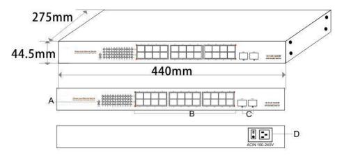
A. Status Indicator B. 24x RJ45 Ports C. SFP Ports D.AC 100-240V,50/60Hz Input
